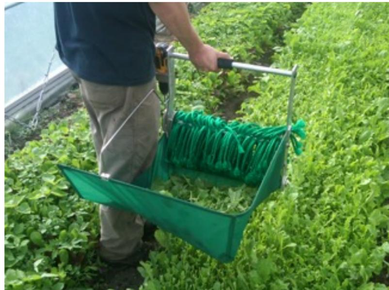
4. **Keep it sharp!** It is critical for proper operation of this product that the blades be maintained and sharpened often. Refer to the **MAINTENANCE** section for in-field sharpening and periodic redressing of blades.
