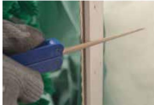
3. **Redressing the blades:** We recommend using a **Work Sharp Tool and Knife Sharpener** to redress the blade. This can be purchased on our website.
